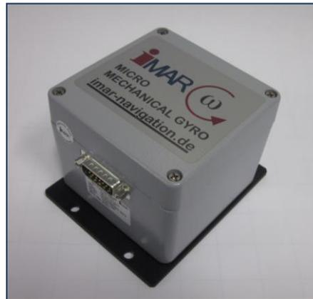
single element followed by high sophisticated analog and digital signal processing. After a high speed digitization and a microprocessor based signal processing the iMGYR-SN provides an output signal being proportional to angular velocity. The integrated micro-processor reduces the non-linearity to much less than 0.2% f.s and compensates the bias on the digital and analog output
